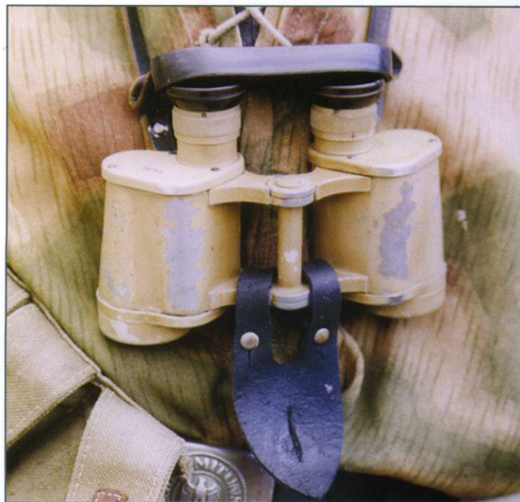
6 x 30 'universal' binoculars (Einheitsdoppelfernrohr) with moulded rubber protective cup and leather flap for securing to a tunic button, in factory finish 'ordnance tan'.
